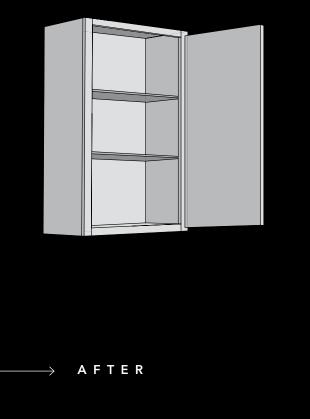
Cut width using door of cabinet. For example cutting a W2430 and still want to use 1 door the width should be 12 1/4" (so you have the 1/4" reveal on both sides)
